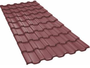
The IBERIC metallic tile is profiled in steel with a thickness between 0.45 and 0.60 mm, zinc-coated (Z225-Z275), covered with a layer of glossy or matte paint. The IBERIC metal tile can be delivered with lengths between 500 mm and 7000 mm.
