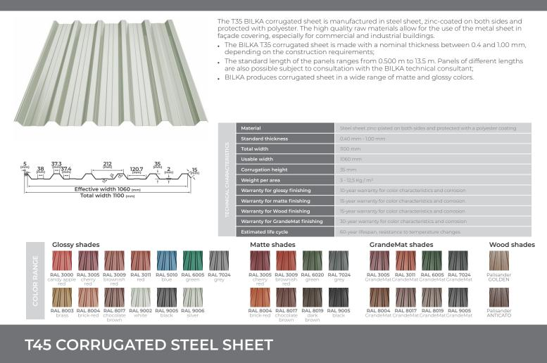
The BILKA T45 corrugated sheet is manufactured in steel sheet, zinc-coated on both sides and protected with polyester. It is used for small inclination roofs and within intermediate floors. It is the ideal and economic solution for the construction and rehabilitation of facilities intended for: warehouses, shopping centers, production facilities, farms, silos, stables, sports centers etc.
