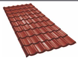
The CLASIC metallic tile is profiled in steel with a thickness between 0.40 and 0.60 mm, zinc-coated (Z225-Z275), covered with a layer of glossy or matte paint. This type of metal roofing is the most widely used, it is similar to classical tiles, and is used especially in residential buildings.
