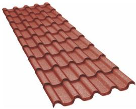
The ROMANIC roof tiles are made of zinc-plated (Z225-Z275) shaped steel sheet with thicknesses between 0.50 and 0.60 mm, coated with a single layer of glossy or matte paint. The ROMANIC metallic roof tiles can be delivered with lengths between 500 mm and 7000 mm.
